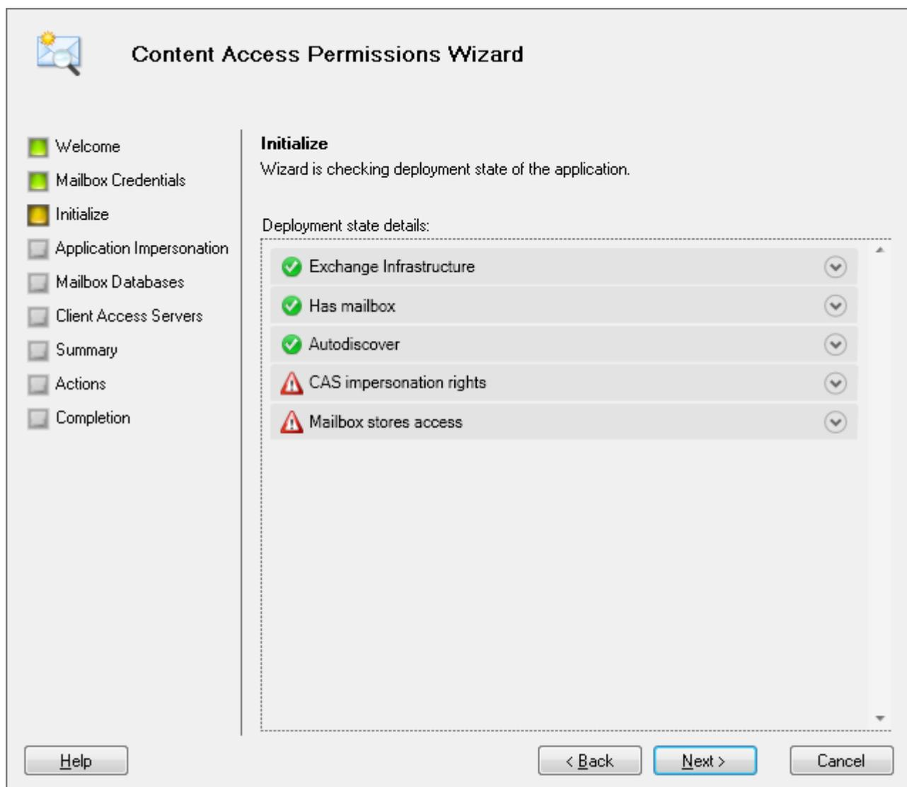
By selecting options with failures, you can get the details and recommendations. The failures can be removed manually or automatically by following the steps suggested by the Wizard.
